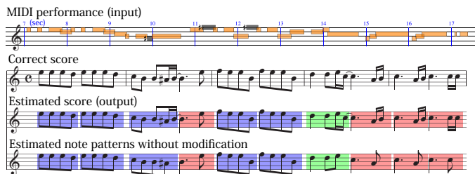
Fig. 5. Example result of rhythm transcription by the proposed model (semi-supervised with modifications modelled). The third low shows the estimated result and the fourth low shows the result after removing modifications.
